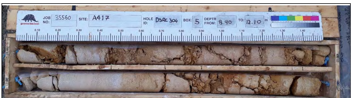
Borehole: DSRCOH304 Box 5: 8.90-12.10m
