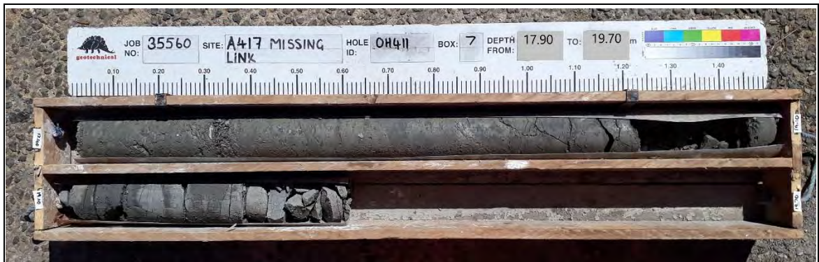
Borehole: OH411 Box 7: 17.90-19.70m
