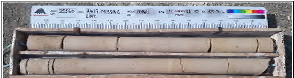
Borehole: OH411 Box 19: 52.70-55.70m
