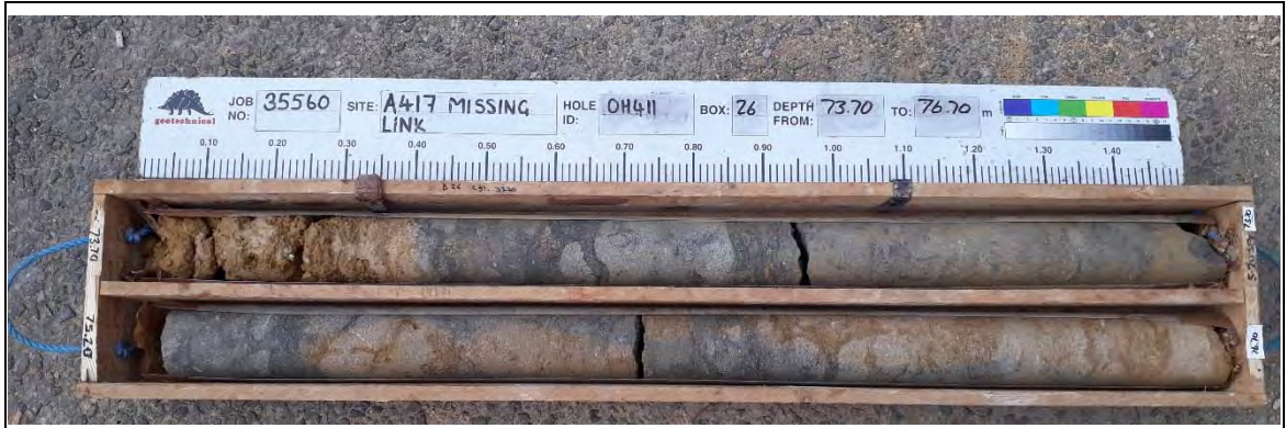
Borehole: OH411 Box 26: 73.70-76.70m
