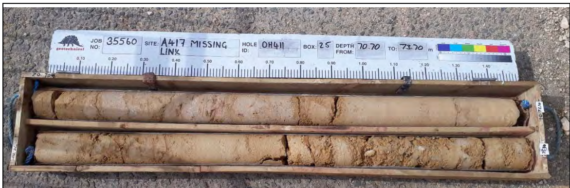
Borehole: OH411 Box 25: 70.70-73.70m
